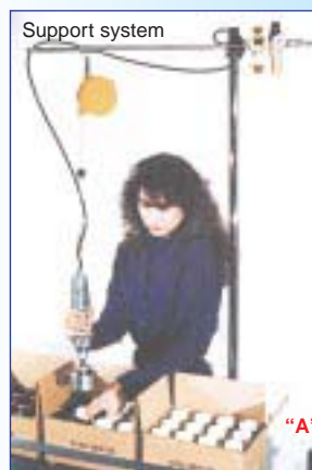
Electronic Machine Torque Monitor shown on Kaps-All's Automatic Cap Tightener
